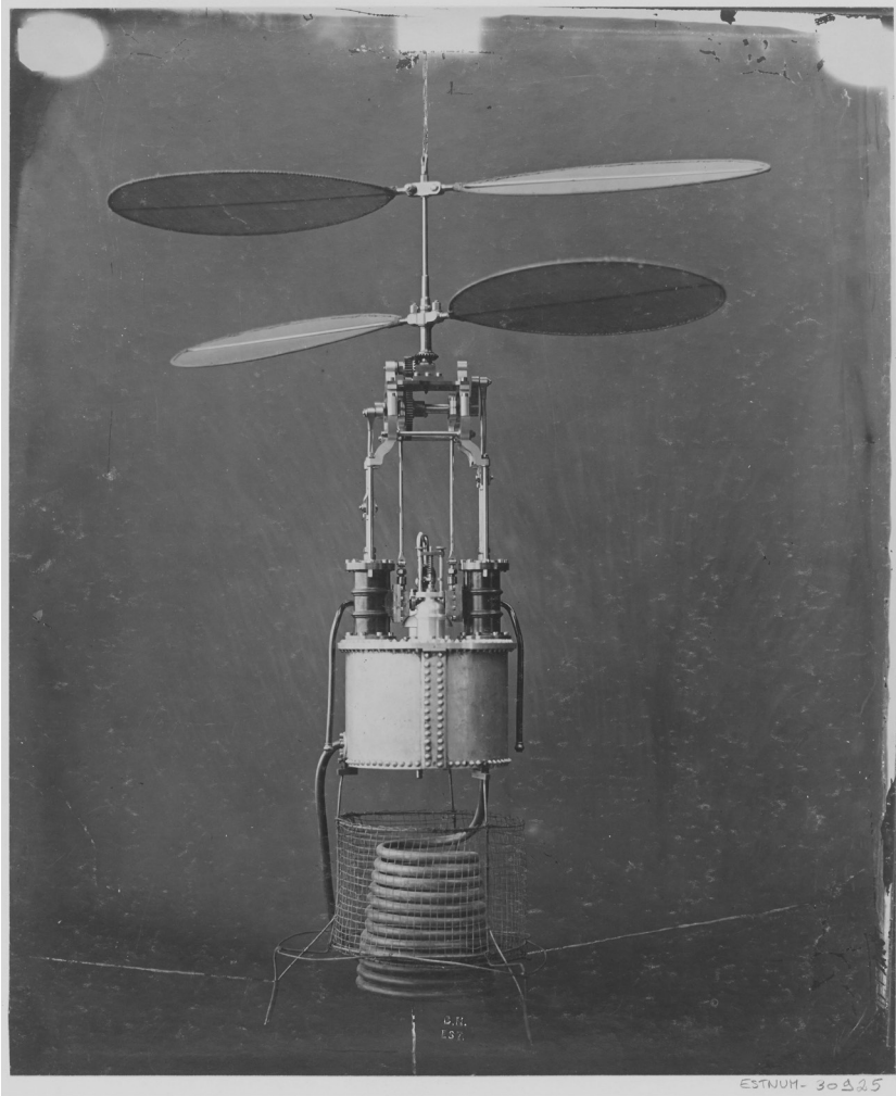
Figure 1.9 Nadar's photograph of one of Ponton d'Amécourt's and La Landelle's helicopters, taken June 1863. 1900 print. Source: gallica.bnf.fr / Bibliothèque nationale de France.
