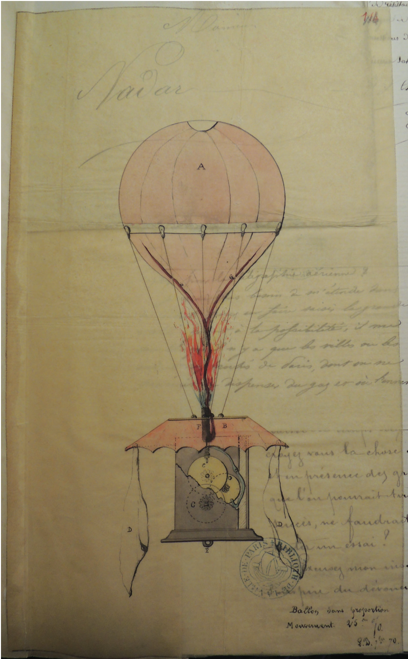
Figure 2.10 Léon Brin's proposal for an automated balloon delivery system to be used to break the Siege of Paris, 9 September 1870. Bibliothèque Historique de la Ville de Paris (MS-NA-471, f. 110).
