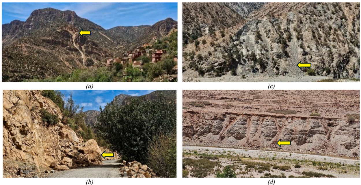
Fig. 7. Earthquake landslide field examples. (a) Mesozoic limestone rockfall with long runout; (b) Mesozoic limestone debris partially blocking the road; (c) Palaeozoic schist rockfalls/slides and soil slide debris runouts; (d) Soil slide failures of Quaternary River terrace sediments.
