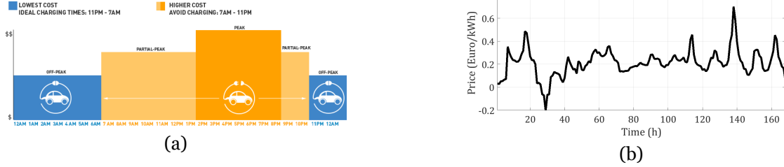
Figure 5. (a) Time-of-Use pricing scheme (source: Pacific Gas and Electric Company). (b) Variable weekly price curve (constructed using EPEX SPOT clearing prices).
