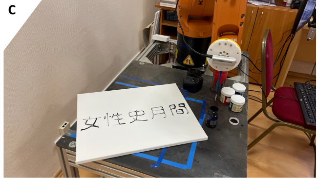
Fig. 5. An example of the skeletonization and painting process. (A) 5 characters form the Japanese term 女性史月間 obtained after translating the Google Trends keyword “Women’s History Month.” (B) The same image after skeletonization of the 2D shapes into 1D curves and conversion from pixels to meters. Different colors represent different strokes in the painting process. (C) An image of the finished painting.
