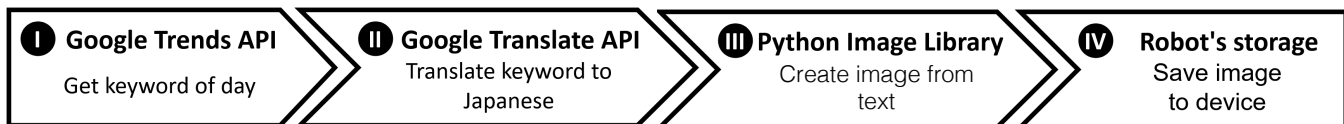
Fig. 2. Workflow for topic selection: Gaka-chu first (I) selects the English keyword with the largest number of searches that day in Google Trends, (II) translates the keyword into Japanese characters, (III) converts the resulting text into an image, and (IV) uses the image as an input for the physical painting process.
