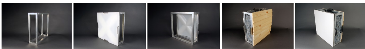
Figure 3. Full scale prototype of a wall module
