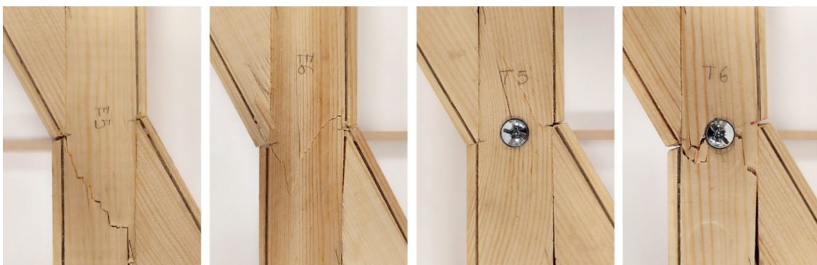
Fig. 13 Details of the failure mode of glued lap and bolted lap specimens with upper notch
