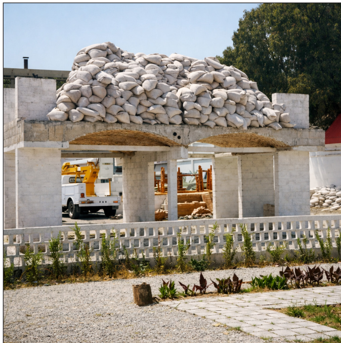
Figure 8: Solutions for vaulted structures at Damascus Expo, 1981: A demonstration and load-testing of shallow vaults from terracotta tubes for floor-systems for rural housing, made by architects from the Faculty of Architecture in Damascus University. Source: Archive of Maen Abaza, 1984.
