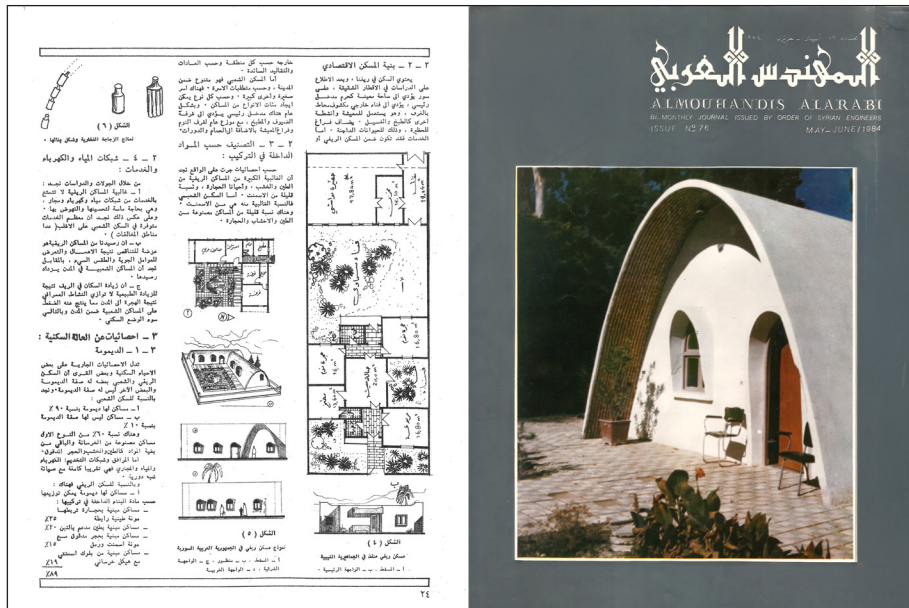
Figure 6: Solutions for vaulted structures at Damascus Expos, 1981: A vaulted rural house as a pavilion in the Expo, on the cover of Al Mouhandes Al Arabi , the monthly journal for Syrian engineers. The vaulted house is made from terracotta tubes developed by Rafee Mouhanna. Source: Archive of Maen Abaza, 1984.
