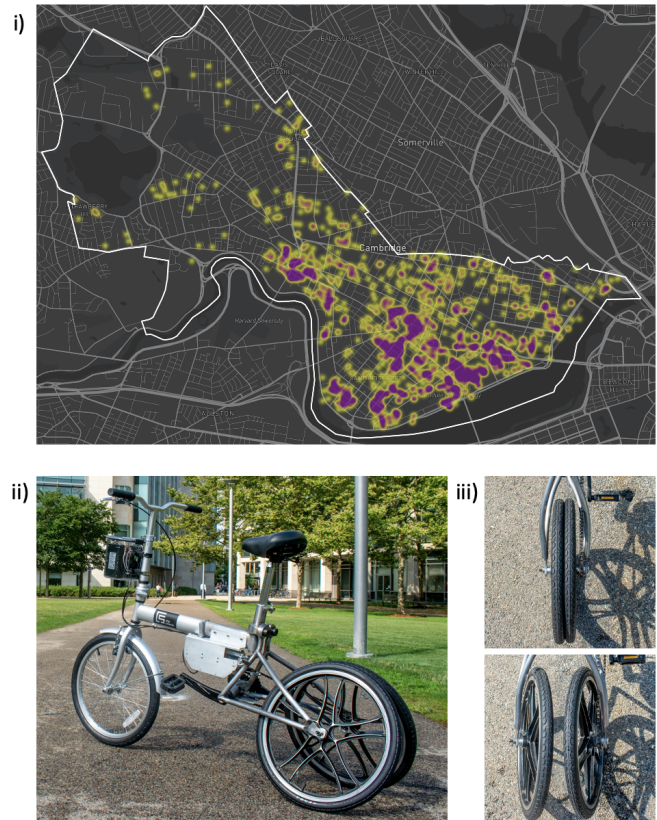
Fig. 5. (i) Heatmap depicting the demand density (highest density areas are shown in violet) and the boundary of the area considered for this study (Cambridge, MA, USA). (ii) MIT Autonomous Bicycle [2], [6], [62], the target vehicle used in this paper and simulated in Sec. III. (iii) Top: Manual driving mode, with the rear wheels folded to act as a single wheel. Bottom: Self-driving mode, with the rear wheels unfolded for stability.
